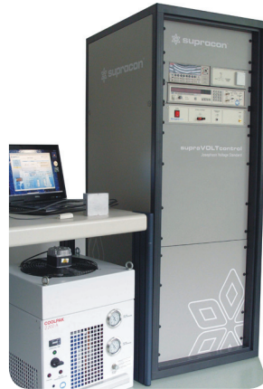
The cryo-cooled Josephson voltage standard, fabricated at Supracon AG Jena / Germany.
