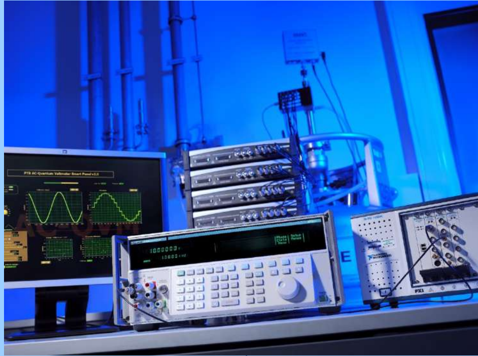
Prototype measurement set-up of the AC Quantum Voltmeter. It is based on a series array of nearly 70,000 Josephson junctions delivering output voltages of up to +/-10 V and is used for calibration of commercially available calibrators [2017].
