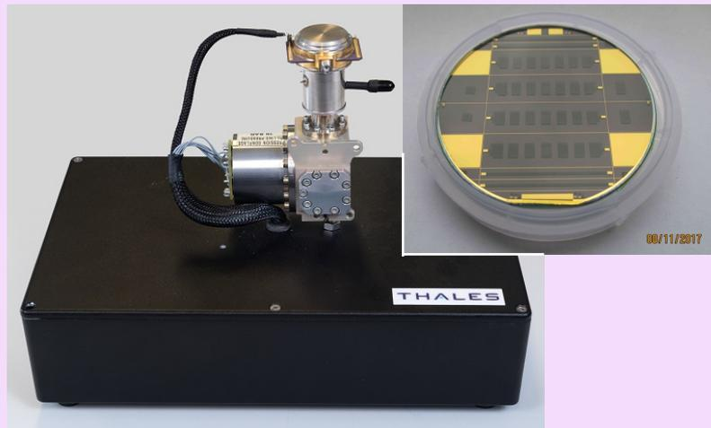
*UHF filter system consisting of a 1cm² HTS chip placed in a sealed vacuum cryostat, cooled by a Stirling rotary machine. The 20cm x 14cm x 5cm black box contains the driving electronics. Right: Four microwave filters on a 2" wafer. Copyright THALES 2009.*
