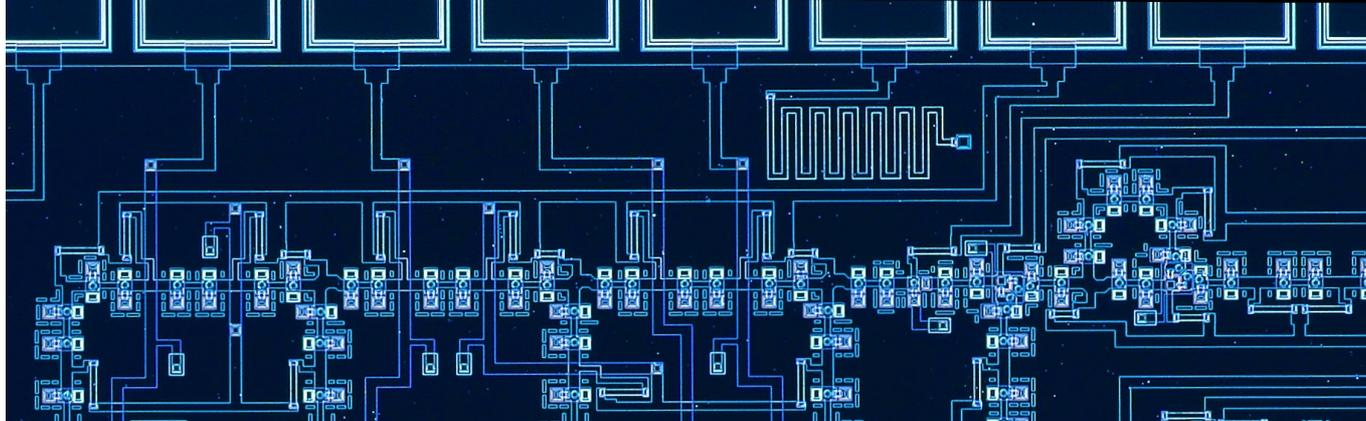
Josephson effect, allowing the quantum-accurate conversion of a frequency into a voltage.
