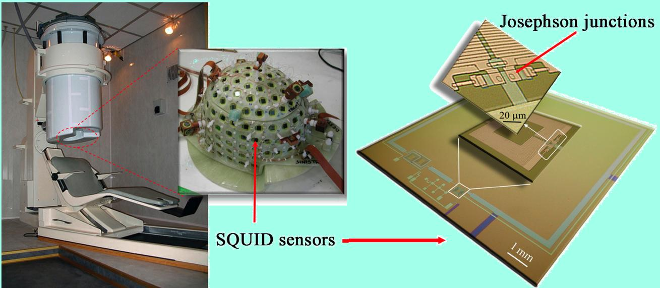
Left: Multi-channel MEG system with 165 sensors operating in a neurological clinic (Hermitage in Naples, Italy)<sup>12</sup>, the SQUID sensors are arranged in a helmet configuration to adapt to the anatomy of the skull. Right: SQUID magnetometer showing a field sensitivity of 1 fT/Hz<sup>1/2</sup>. The outer square loop transduces the field into magnetic flux in the SQUID with its depicted Josephson junctions.
